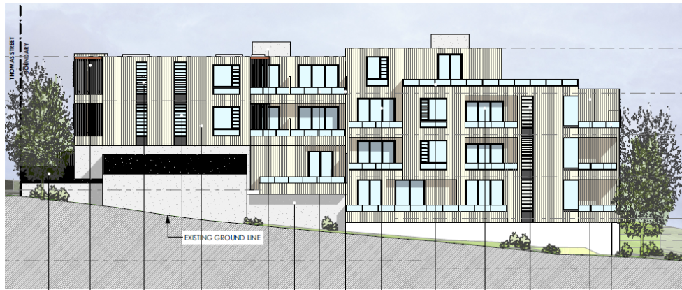
Figure 7: Extract of southern (side) elevation exemplifying how the built form 'steps down' the site's gradient towards the Parramatta River (Source: PTI Architects)
